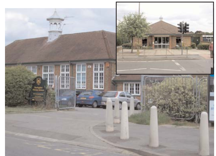
The bollards establish basic safety, however softer design measures such as raised kerbs or the use of different pavement material could enhance the pedestrian environment.
